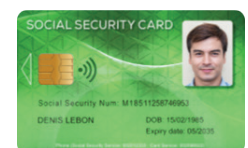
Card printed with new YMCKOO ribbon after 300 abrasion cycles (Taber test)
