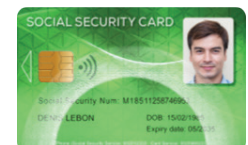
Card printed with standard YMCKO ribbon after 300 abrasion cycles (Taber test)
